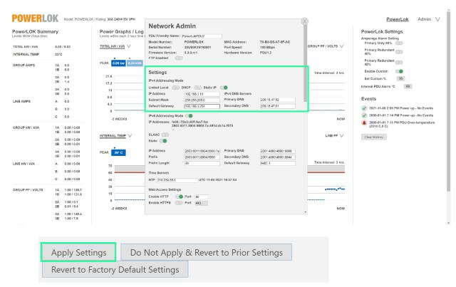
This should complete the necessary steps to configure for the router. Connect the PDU to the router, open a browser and enter the static IP address to access the PowerLok web server.
